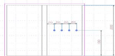
Fig 2: Transverse position of thermocouple
