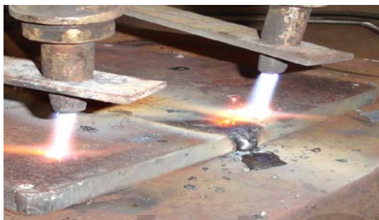
Fig 4: moving heat flame mechanism
