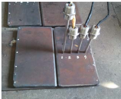
Fig 5: Transverse position temperature Measurement
